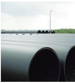
Dia. 1,400 mm PE pipes in the factory in Kleszczów.
